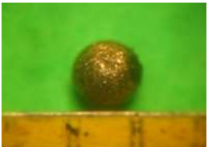
Approximately 500 gm rock sample produced 1 mm sphere of metallic gold.
