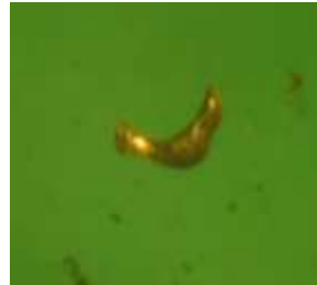
1 Kg Quartz Sericite Schist, crushed, panned, produced free 2 gold particles and spheres of PGE oxide, and gold.
