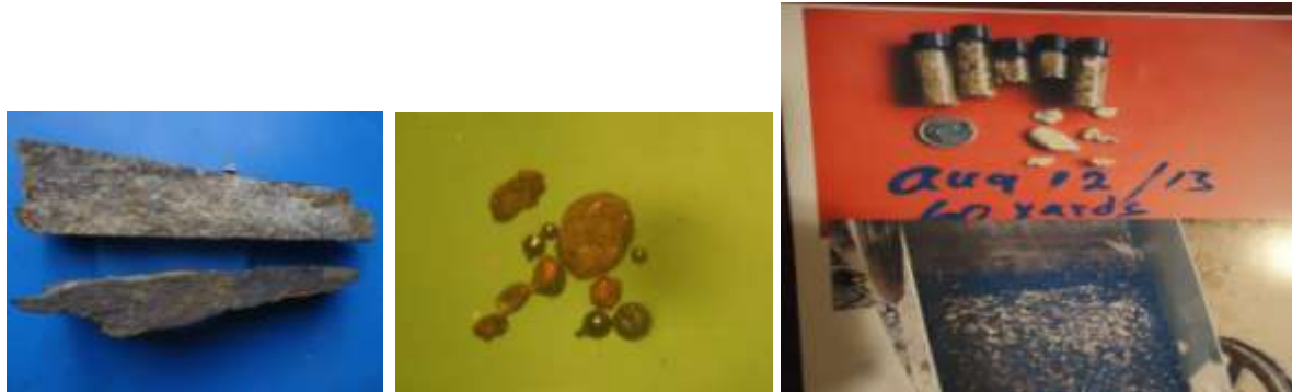
Talus 290 gm, crushed, panned: Produced Free Cu & Au/PGE 60 cu.yrd. of Talus produced 10 oz.
