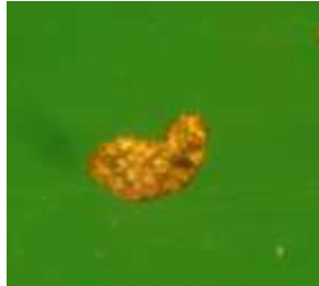
1 Kg Quartz Sericite Schist, crushed, panned, produced free 2 gold particles and spheres of PGE oxide, and gold.
