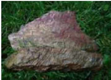
1 Kg Quartz Sericite Schist, crushed, panned, produced free 2 gold particles and spheres of PGE oxide, and gold.
